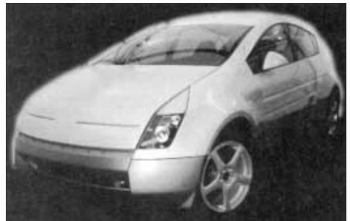
**Hypercar, powered by a fuel-cell, zero-emission engine takes oxygen from the air and hydrogen from its tank to create a chemical reaction that produces electricity and water—the only by-product is developed by the Rocky Mountain Institute.**
